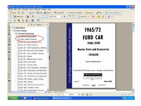
Step #2 – Click on the alphabetical index under the letter "P" for the word "plate". Under the letter "P" in the index, scroll through the entries until locating "Plate (rear brake backing)". The group number listed is for the part is 2211-2.
